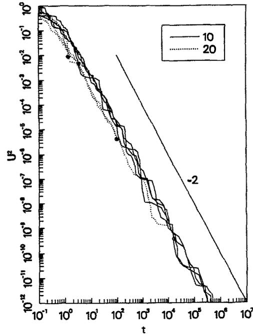
FIG. 4. The mean square velocity as a function of time for a cooling inelastic gas with  $r = 0.8$ . We show four realizations with  $N = 10$  and 20. The  $t^{-2}$  regime is clear for realizations with  $N = 10$ . But in the other cases, the  $t^{-2}$  regime is transient and is halted by inelastic collapse (indicated by the heavy dots).
