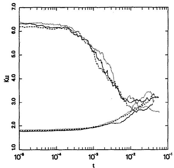
FIG. 9. The kurtosis, defined in Eq. (10), as a function of time for six realizations of the  $r = 0.8$  and  $N = 1000$  inelastic gas. The three simulations that begin with  $Ku \approx 1.8$  are the three simulations in Fig. 6. The other three have a piecewise constant initial velocity distribution, constructed to give  $Ku \approx 6$  and  $U^2 \approx 1$ . By collapse time, all six realizations are close to the Gaussian value  $Ku = 3$ .
