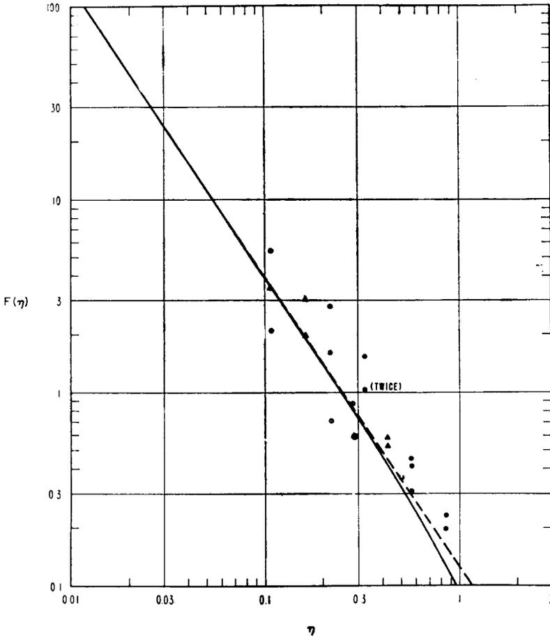
Fig. 7. (from LONGUET-HIGGINS and STEWART, 1963). The non-dimensional form of the wave set-up outside the breaker zone, compared with the observations of SAVILLE (1961).
