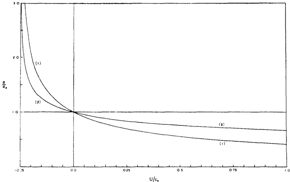
Fig. 12. (from LONGUET-HIGGINS and STEWART, 1961). The relative amplitude of waves propagated on a steady, non-uniform current  $U$ , (1) with upwelling from below (2) with horizontal inflow from the sides.
