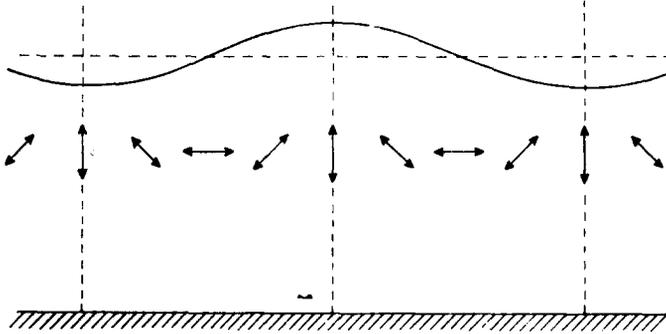
Fig. 4. Particle velocities in a standing wave. The components  $u$  and  $w$  fluctuate in-phase, and the mean product  $\overline{uw}$  is non-zero in general.
