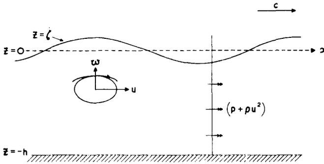
Fig. 2. The momentum flux in a progressive wave.
