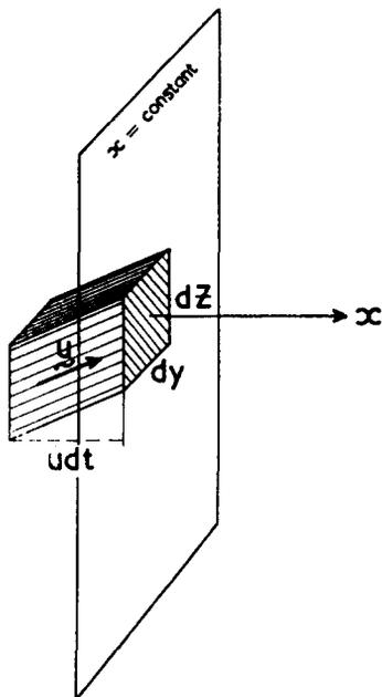
Fig. 3. Bodily transport of momentum across a plane  $x = \text{constant}$ . In time  $t$  a volume  $udt$  per unit area has been transported across the plane. The momentum transported is thus  $\rho y u dt$ .
