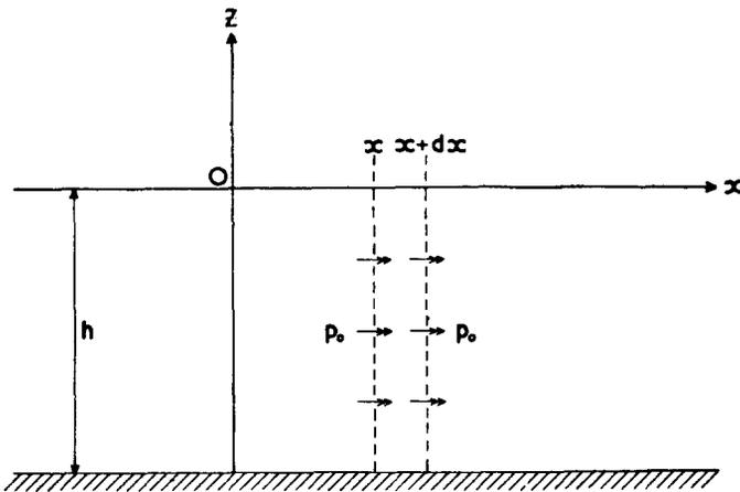
Fig. 1. The momentum flux in a stationary fluid.
