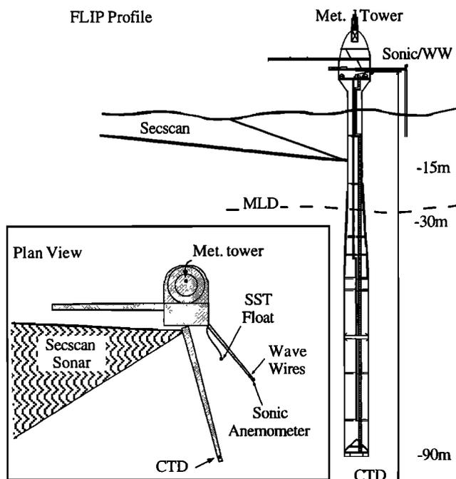
**Figure 2.** Plan and profile views of *Flip*, MBLEx leg 1, showing various instrument locations. The phased array and SW sonars were mounted on an active heading compensation system, maintaining bearing to within 0.1° rms.
