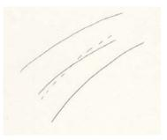
When the data line coincides with a characteristic, the solution is *overdetermined* along that characteristic, and *undetermined* everywhere else. In that case we have two choices:
