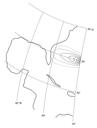
Figure 14. The sea-surface elevation west of 70W in solution WWG25, with Green's function boundary condition (5.1), no local wind forcing, and  $\epsilon/\beta = 25$  km. Contour interval, 11.2 cm. "Beta advection" carries the high surface pressure directly westward to the North American coast.
