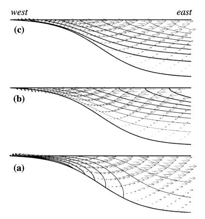
Figure 3. East-west sections of  $\phi$  at (a)  $y = \frac{1}{6}$ , (b)  $y = \frac{1}{2}$ , and (c)  $y = \frac{5}{6}$  in the same solution as in Figure 2. These latitudes correspond to the three bottom-velocity extrema in Figure 2d. Darker contour lines correspond to larger values of pressure. The arrows represent the velocity tangent to the section.
