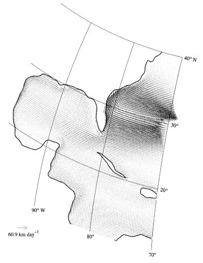
Figure 15. The horizontal velocity at the ocean surface in the same solution (WWG25) as Figure 14. The arrows are proportional to the *square root* of the fluid speed. The longest arrow on the diagram (which has the same size as the arrow at the lower left) corresponds to the maximum velocity of 60.9 km day<sup>-1</sup>.
