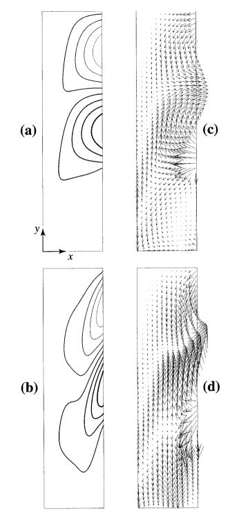
Figure 5. The same as Figure 2, but with a larger  $\kappa = 10$  and the *z*-independent open-boundary condition (3.23). The flow has begun to resemble the depth-independent flow depicted in Figure 1d for the case of homogeneous fluid, which corresponds to the limit  $\kappa \to \infty$  in (3.3).
