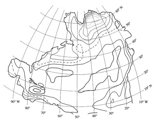
Figure 8. The quantity  $f\delta_E W_s$ , which, away from the equator, approximately equals *minus* the wind stress curl.  $W_s$  is the surface value of the "source term" W in the  $\phi$ -equation (2.5). Darker contours correspond to larger values of  $W_s$ , and the zero contour is dashed. Contour interval,  $4.0 \times 10^{-5}$  km day<sup>-2</sup> (equivalent to  $5.2 \times 10^{-10}$  cgs). Note the large positive source in the eastern Caribbean.
