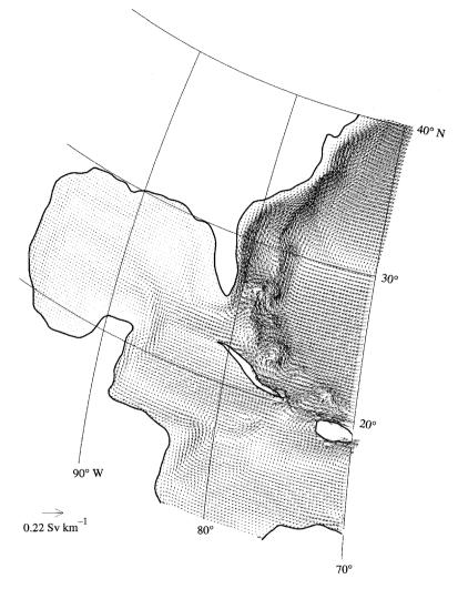
Figure 25. The vertically integrated horizontal velocity in solution WW25, which has no wind forcing west of the heavy line in Figure 7. Maximum transport, 0.22 Sv km<sup>-1</sup>.
