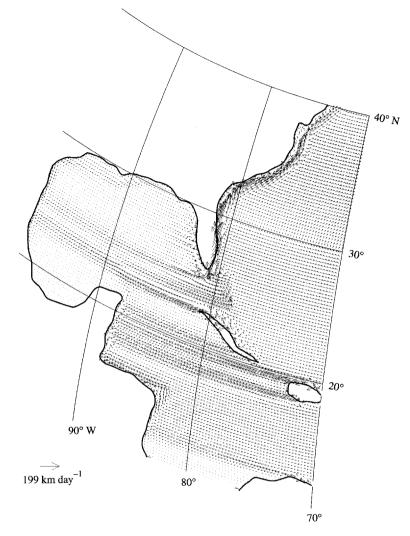
Figure 21. The horizontal velocity at the surface in the solution WW1 with friction parameter  $\epsilon/\beta = 1$  km, no local wind forcing, and open-boundary condition of pressure  $\phi$  equal to that of the full-basin solution FB. Maximum velocity, 199 km day<sup>-1</sup>. At this low value of friction, and with no local wind forcing, the islands and Great Bahama Bank cast long "beta shadows," with internal boundary layers of high surface velocity at the edges of the shadows.
